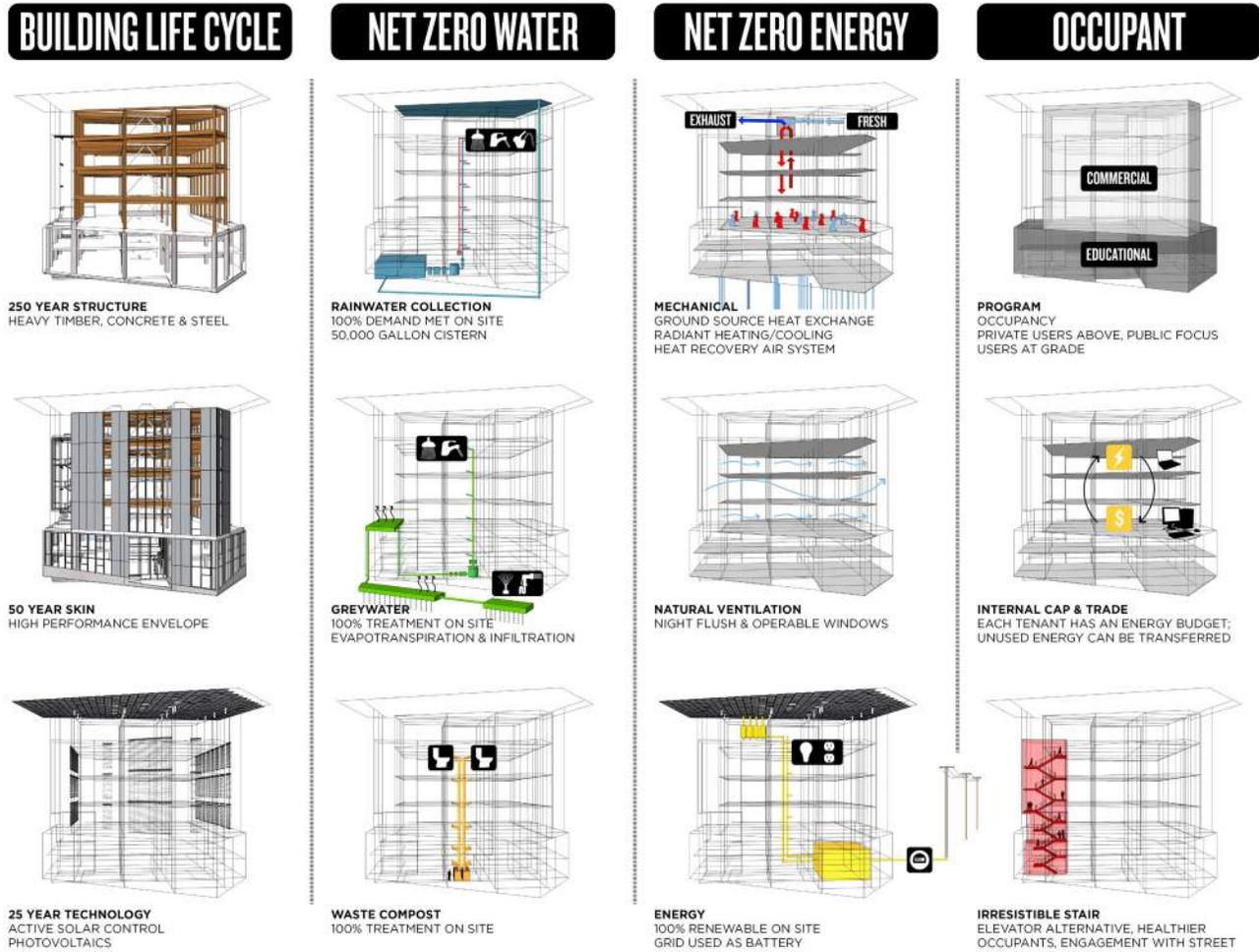
Figure 15. Integrated Design elements of the Bullitt Center (Miller Hull).
