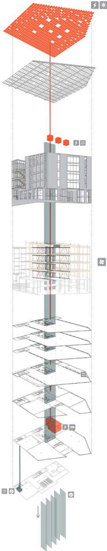
Figure 19. Exploded view of the primary elements of the buildings energy supply and energy efficiency measures.
