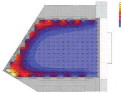
Figure 28. Daylight distribution (measured in daylight factor) for an 14'-2" floor-to-floor height.
