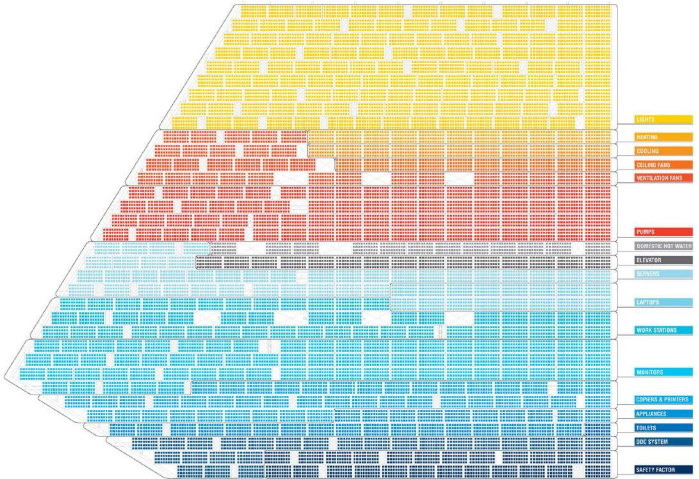
Figure 40. Plan of the PV array illustrating the proportion of array devoted to various end-uses; blue and gray are all “activity” loads.
